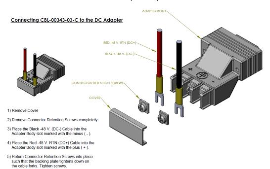
Install the Adapter on the ND2340-01 power supplies and connect the common ground cable to the chassis ground lug.
