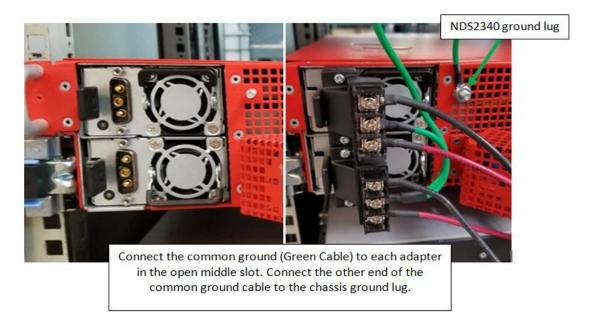
Installing the Adapter on the NDS1080-01 power supplies is similar to the NDS2340-01. The
